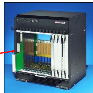
Carrier blades in ATCA chassis
